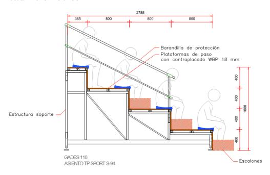
Removable tribune assembled through steel screws with a minimum platform of 800mm. Prepared to fit individual seats model TP SPORT S-94 SG on the top of the platform through screws.
