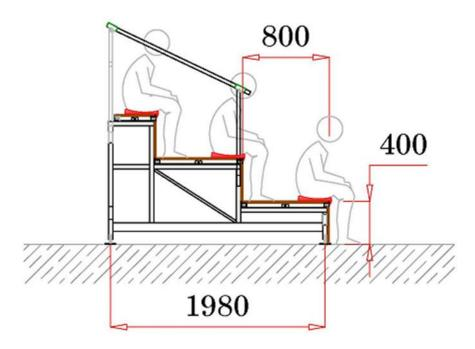
Fixed tribunes assembled through Steel screws with a minimum platform of 800mm. With TP SPORTS seats S94-SSG attached to the top of the platform through screws. Legs fixed on the ground to ensure complete fixation. It is supplied by pieces and they are assembled through steel screws.
